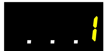
Multi-function Output Terminal "Y1" is active
