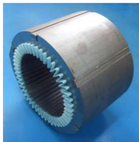
Figure 4-2: Stator core with winding
