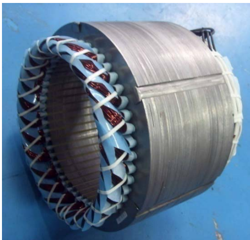
Figure 4-1: Stator core with slot liners
